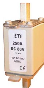
NV TELECOM fuses have been available only in the standard size **NV00** for the voltages up to **80 V DC** and nominal currents from **160A** to **800A**. According to IEC, the highest allowed current in size NV 00 is  **$I_n = 160A$**  and the maximum allowed nominal power  **$P_n = 12W$**  (see IEC 60269-2, Ed.3, 11/2006).
